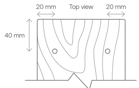
The length of screws or nails should be at least 2.5 times the thickness of the board at its thickest point.
