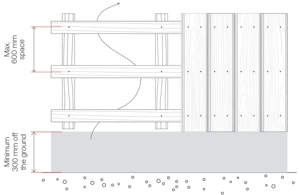
Fix **vertical cladding** onto horizontal battens; the joint ends of the boards must be resting on the battens with standard cladding boards. Joint end-matched boards can be placed
