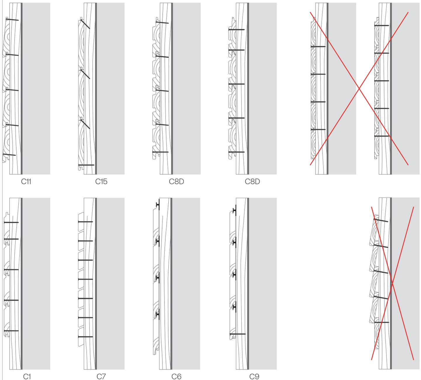
For shiplap profiles, leave an air circulation space of 2-3 mm to allow for swelling of the wooden boards.
