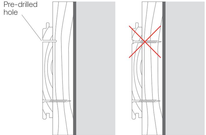
**THERMORY CLADDING PROFILES FOR FASTENING WITH SCREWS, STAPLES OR NAILS:**
